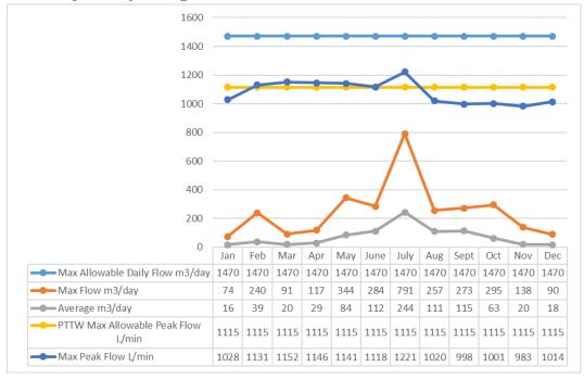
The above table shows there were spikes in <u>instantaneous</u> peak flow rate (L/min) and max flow rate these occurrences were caused during pump start-up/pump to waste. The increased flow rate seen in July was due to maintenance.
