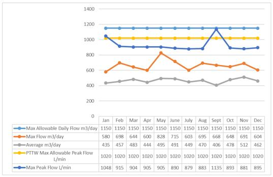
The above table shows there were spikes in <u>instantaneous</u> peak flow rate (L/min) and max flow rate these occurrences were caused during pump start-up/pump to waste.
