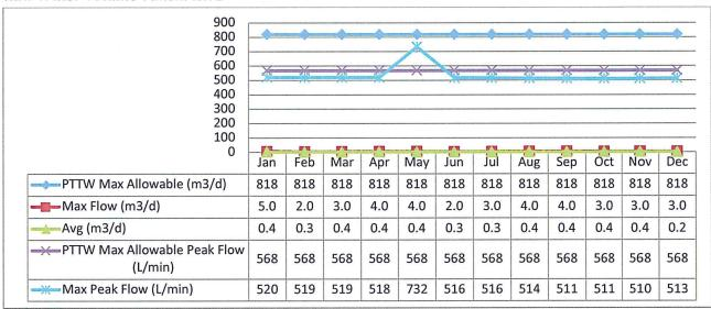
May 2016 - PTTW Max allowable peak flow was exceeded due to Annual Flow meter calibrations
